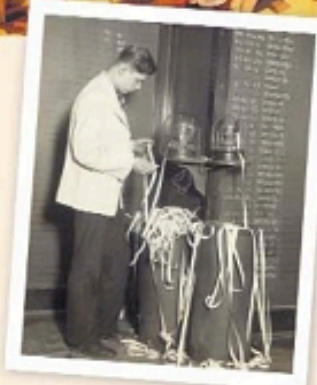
Before the days of computer technology, ticker-tape machines were used to punch the stock prices onto paper strands.
